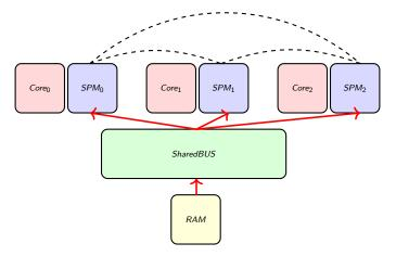
→ = Memory Transfer (RAM to SPMs) via Bus --- = Data Transfer (Inter-SPM Communication)
